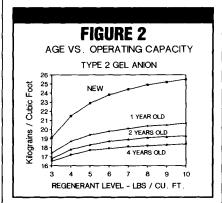
working mixed bed demineralizers. The data is presented in a manner that shows the percentage of the original operating capacity that each anion resin retains as its age and service increases. Each figure has separate curves for different bed heights, as you can see
