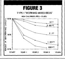
mixed beds can be sensitive to bed height. The data in Figures 3 and 4 are based on operating flow rates of two gallons per minute per cubic foot. Figure 5 shows four-year projections of the relative performance of a Type 2, compared to a Type 1, resin in mixed beds of various depths.
