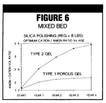
seeing high chloride waters and where the anion resin is regenerated at eight pounds per cubic foot.
