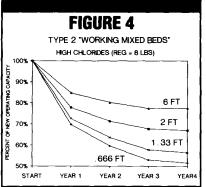
a much higher level. Below two feet, the bed depth capacity loss is quite noticeable for both kinds, but more severe for the Type 2 anion resins. Changing the flow rate changes the polishing zone height and the percentage utilization, in a manner similar to changing the bed height. As anion resins age, their functionability changes, and
