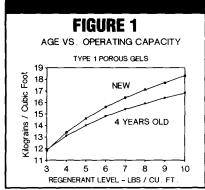
2 anion resins in separate bed service on a high chloride water. In this case the Type 2 resin gives the most capacity. A Type 2 will always start off with a higher capacity, it also tends to lose it more rapidly than the Type 1, but still retains its advantage. The rate of loss depends on the regenerant level and water analysis. Generally speaking, on a long-term basis,
