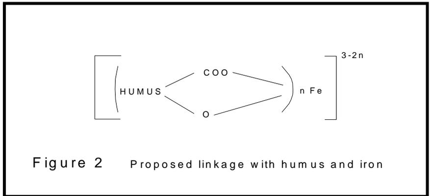
Cleaning organically fouled anion resin requires time, elevated pH, and is helped by high temperatures. The organic ions are slow-moving and require more time than standard ions for elution, and the organic acids are more soluble at a higher pH. Also, higher temperatures increase the rate of reaction.
